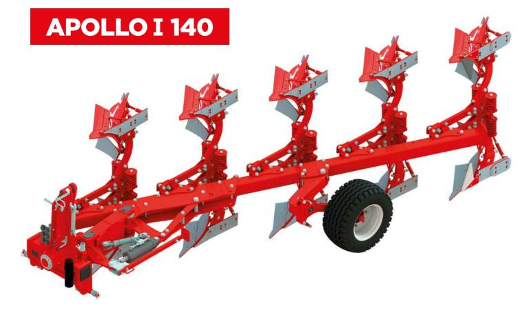
APOLLO I models are four- to six-plough bodied mounted reversible ploughs designed for tractors from 120 horsepower. Adjustment of plough bodies width is performed mechanically by changing the position of the plough body holder on the plough frame.
