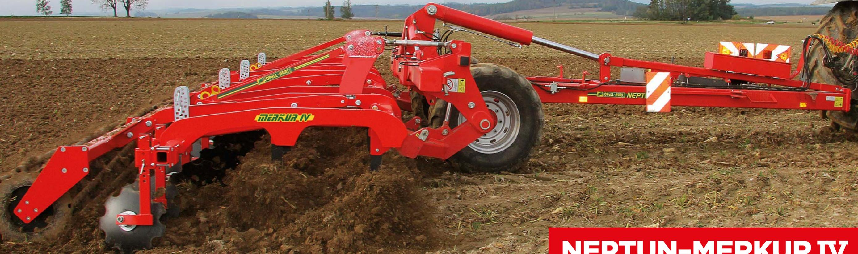
The NEPTUN-MERKUR IV cultivator is designed for soil cultivation after the harvesting of cereals and preparation for harvesting of the intercrop. It is also suitable after harvesting sugar beet, corn and pre-crops when there is not enough time for classic ploughing.
